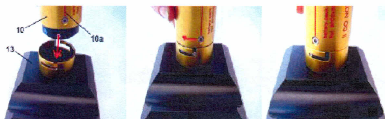
Fig. 6 Putting the battery cartridge in the charger support unit
