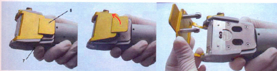
Fig. 13 Opening the cover for access to the blade compartment
